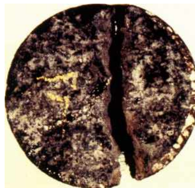
A core sample of a water-effected pavement surface showing extensive cracking. Crack Sealing, using appropriate and suitable products, will prevent these types of situations, if treated early enough. Crack Sealing with SAMIfilla HM seals the crack/joint and keeps water out.
